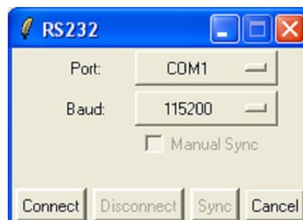
7. Click **Connect** button to communicate with MCU in Monitor Mode and it will display result as the picture below.
